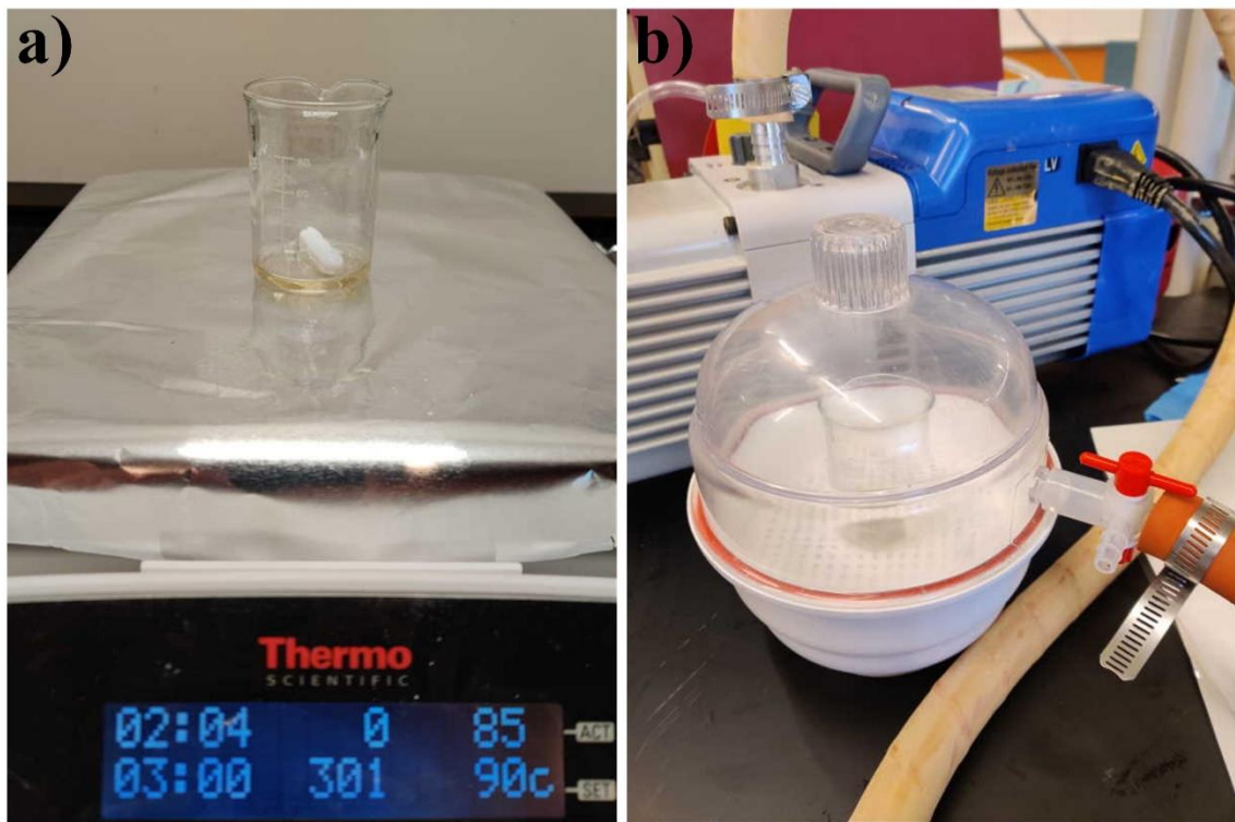
Figure 22. a) Evaporation of solvents from the PVDF/ZnO solution. b) The PVDF/ZnO solution in a de-bubbler after the evaporation process.
